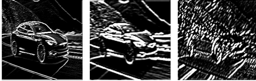
Figure 14: Features extracted from an image of a car by the layers of a trained VGG model. Left: Low-level features from early layers - lines and edges. Middle: Mid-level features from layers in the middle - textures and shapes. Right: High-level features from deeper layers - door, window and wheels.
